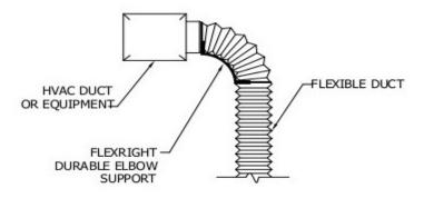
NOTE: INSTALL FLEXRIGHT DURABLE ELBOW SUPPORTS AT ALL FLEXIBLE DUCT 90° BENDS.
