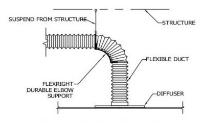
NOTE: INSTALL FLEXRIGHT DURABLE ELBOW SUPPORTS AT ALL DIFFUSERS.
