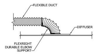
NOTE: INSTALL FLEXRIGHT DURABLE ELBOW SUPPORTS AT ALL DIFFUSERS.
