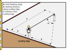
Starting calculation point for determining correct anchorage positioning must be directly in-line with standing seam on which 2-Way Standing Seam Clamp is installed.
